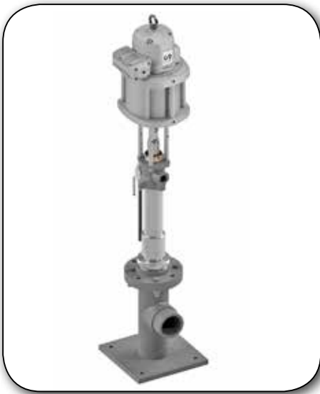
PM80 20:1 ratio Dynamic-Primer pump for extruding heavy materials, flange mounted to a floor suction stand.
