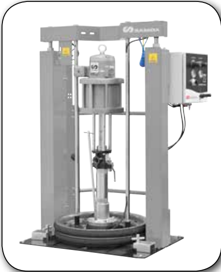
PM80 50:1 ratio Dynamic-Primer pump for extruding heavy materials mounted on double post air operated inductor plate.
