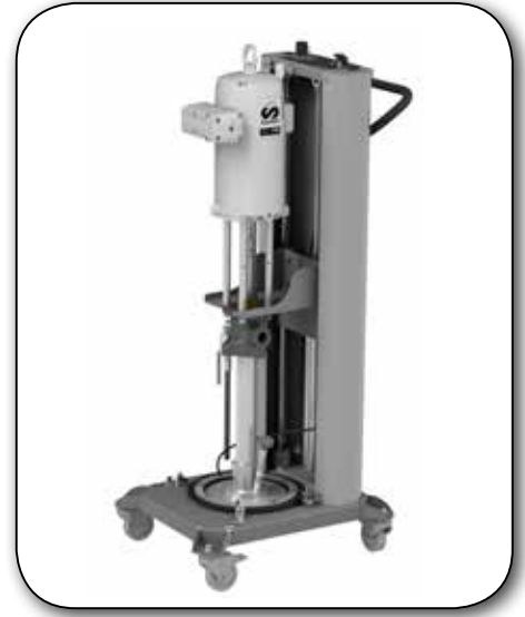
PM45 40:1 ratio Power-Piston pump for extruding heavy materials mounted on an air operated mobile inductor plate for 20 kg pails.
