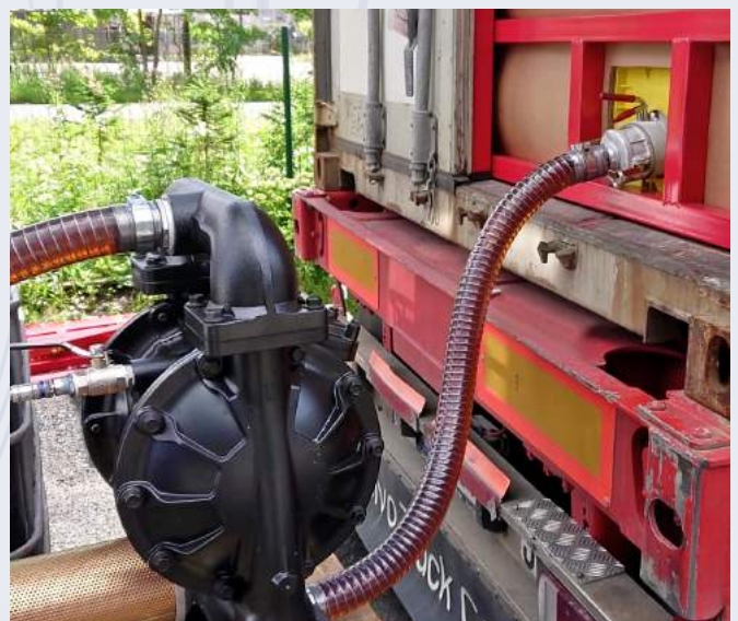
High fluid viscosity reduces pump delivery.
