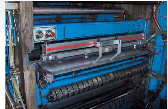
Version BIA-PSH pneumatically driven ink agitator with blades, provided for installation on top of the ink leveler
